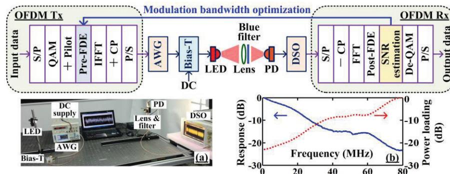
Fig. 1. Experimental setup. Insets: (a) photo of the overall system and (b) frequency response and power loading coefficients of pre-FDE.
