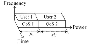
Fig. 1. Conceptual diagram of power domain energy-efficient NOMA.
