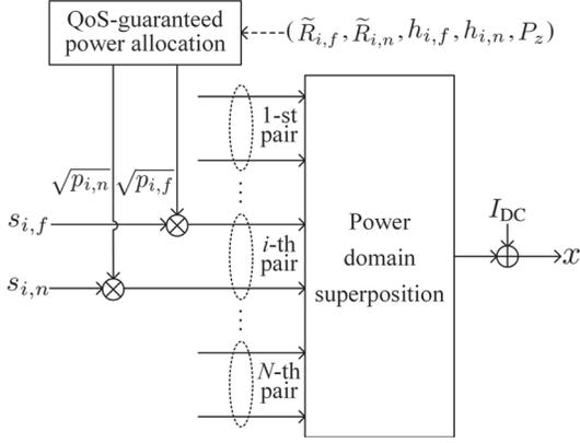
Fig. 2. Schematic of energy-efficient NOMA-enabled multi-user VLC.
